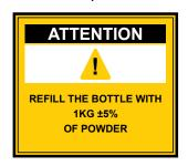
As extinguishing agent, use only the extinguishing powder mentioned in Part 4 of the label (cfr following image).
